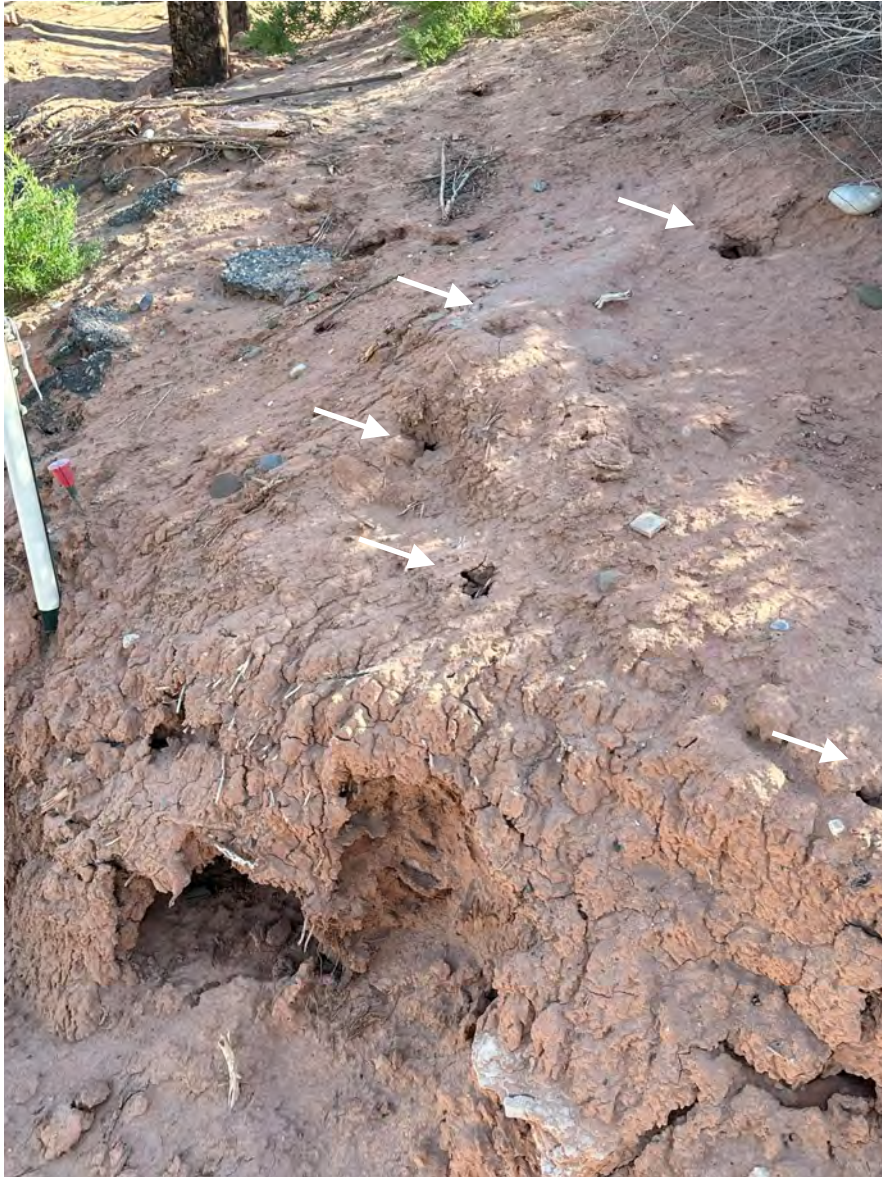
Small openings ('swallow holes') in upper unexcavated slope are entrances to eroded pipe-like openings within sediment ('piping')
